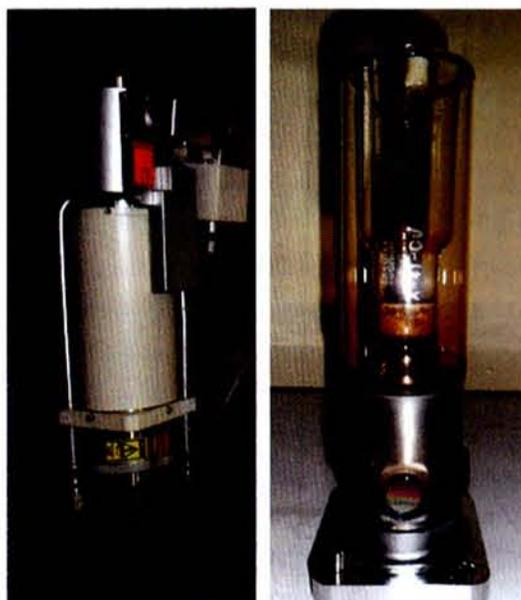
Fig. 2: X-ray Tube Holder and X-ray Tube
