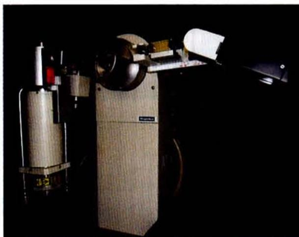
Fig. 1: Rigaku Multiflex 2KW Powder X-ray Diffractometer at URC-YU
